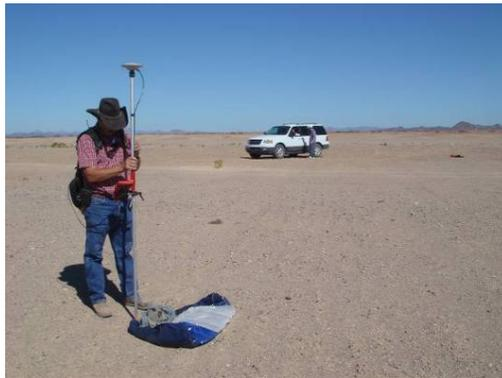
**Fig. 17** Geodetic survey of the touchdown point.
