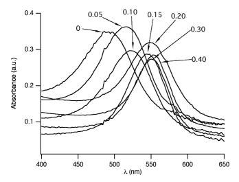
Figure 2. Absorbance spectra of individual LCDs prepared with 2 and varying equivalents of 4a. In all cases, the LCDs were prepared as a blend with 5.4 mol. % 2, 37.2% cholesteryl chloride and 57.4 mol. % cholesteryl pelargonate. The absorbance measurements were referenced to an air background.
