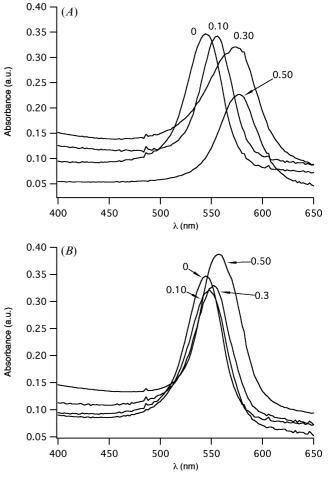
Figure 4. Absorbance spectra of individual LCDs prepared with 2 and varying equivalents of neutral guest molecules. In all cases, the LCDs were prepared as a blend with 2.0 mol. % 2, 39.0% cholesteryl chloride and 59.0 mol. % cholesteryl pelargonate. The absorbance measurements were referenced to an air background. (A): guest 4a; (B): guest 4c.
