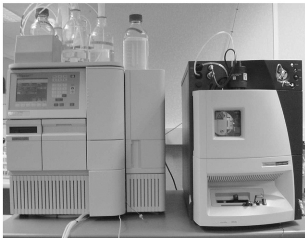
Fig 1. Tandem mass spectrometer. Reprinted with permission from Waters Corporation (MS Technologies Centre, Milford, MA).
