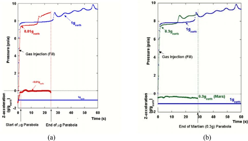
Fig. 4: (a) Comparison of pressure histories obtained at reduced-gravity (KC-135 aircraft) and 1g and (b) Martian gravity versus 1g for nearly identical initial pressures at  $T=320^\circ C$ . The 1g data is the same in both (a) and (b). Mixture composition is  $C_3H_8:O_2$  (1:1). The vertical component of acceleration is shown in the lower portion of the plot (negative value indicates downward acceleration).
