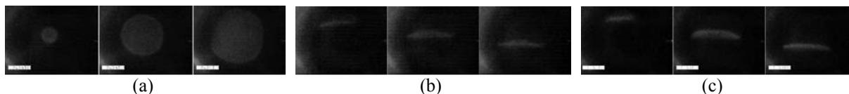
Fig. 5: Representative cool flame images in  $\text{C}_3\text{H}_8:\text{O}_2$  at  $320^{\circ}\text{C}$ , 10.2cm i.d. quartz vessel at (a)  $\mu\text{g} \sim 10^{-2}\text{g}$  (12.0 psia), (b) 0.3g (7.6psia), and (c) 1g (7.8psia). Time lapse between sequential images in 1/3s. Images have been enhanced for clarity.
