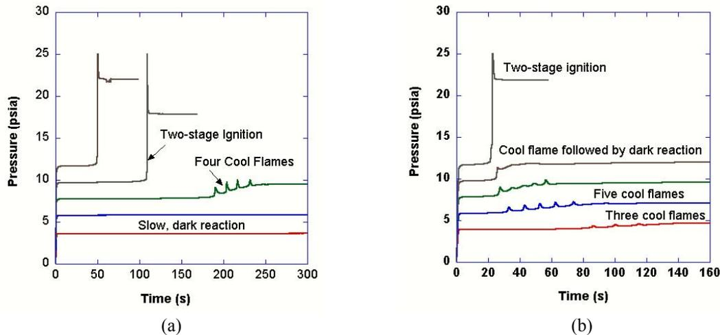
Fig. 2: Pressure histories at 1g at (a)  $T=310^{\circ}\text{C}$ , (b)  $T=320^{\circ}\text{C}$  for five experiments at different initial pressures. Mixture composition is  $\text{C}_3\text{H}_8:\text{O}_2$  (1:1).
