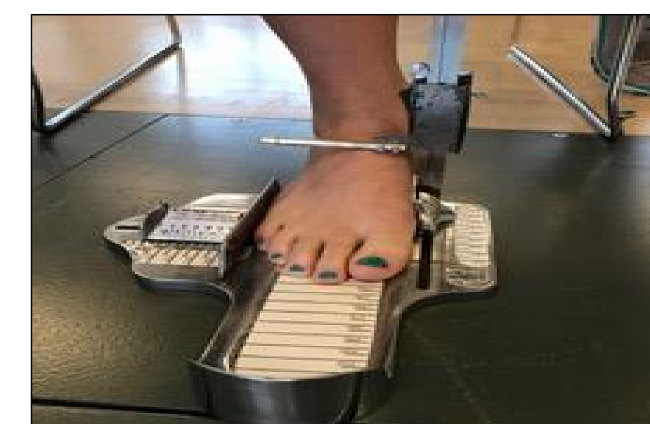
Picture 6: Arch Height Index Measurement Device, anterior view of right foot from seated position
