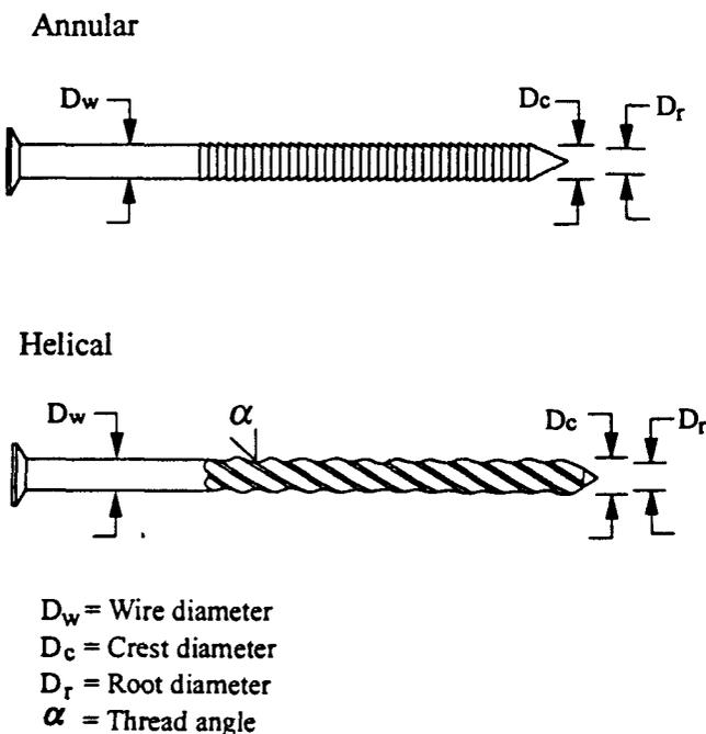
**Figure 1—Dimensions of helical threaded-shank and annular threaded-shank nails. Thread expansions are equal to thread depressions for helical threads, therefore the effective wire diameter remains the same. However, with annular threads the effective diameter (root diameter) is less than the initial wire diameter.**
