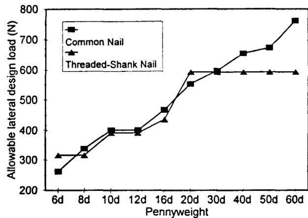
Figure 2—Comparison of lateral design values for different pennyweight designations, based on 12.7 mm (1/2 in.) side member thickness and a specific gravity of 0.50 (AF&PA, 1991).
