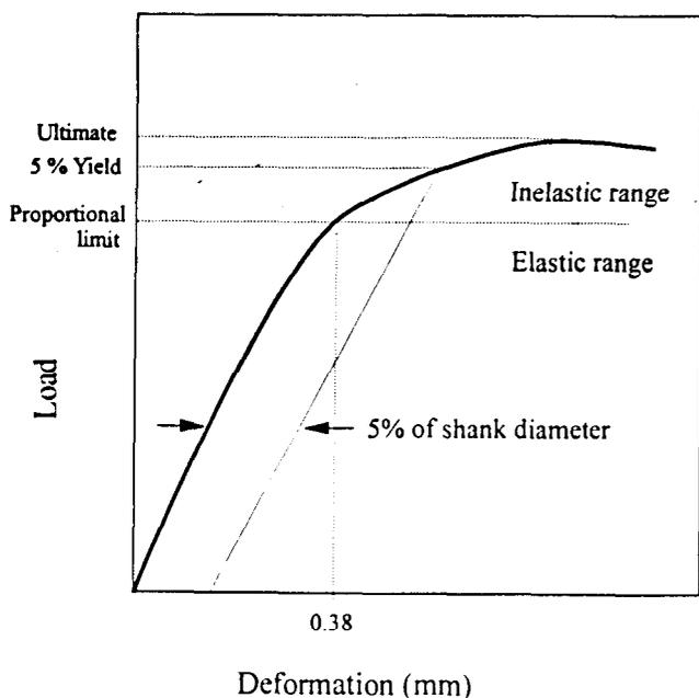
Figure 4—Comparison of load at 0.38 mm (0.015 in.) proportional limit, 5% offset yield point and ultimate capacity (Winistorfer, 1992).
