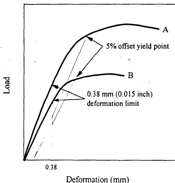
Figure 5—Comparison of proportional limit at 0.38 mm (0.015 in.) deformation vs. 5% offset yield point for two nailed connections. The 5% offset yield is a better indicator of nail performance.
