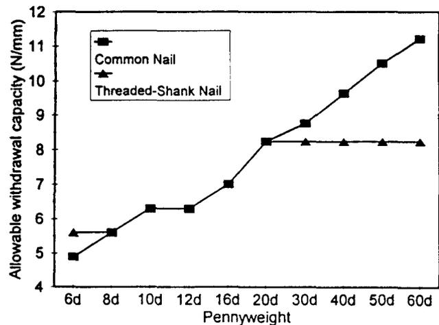
Figure 3—Comparison of withdrawal capacities for different pennyweight designations, based on a specific gravity of 0.50 (AF&PA, 1991).
