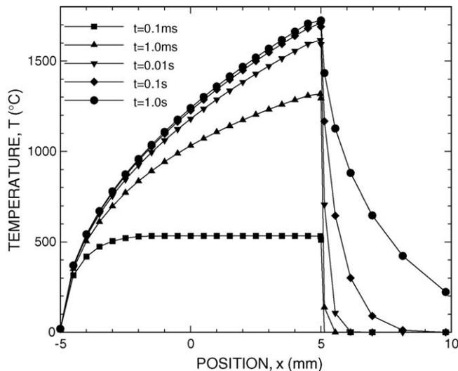
Fig. 3. Temperature distribution along the contact patch at various times.
