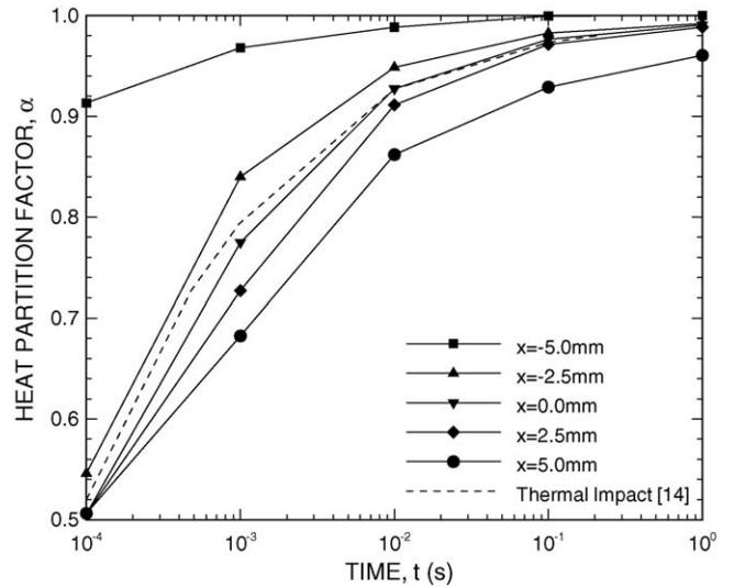
Fig. 4. Heat partition factor vs. time at various positions along the contact patch.
