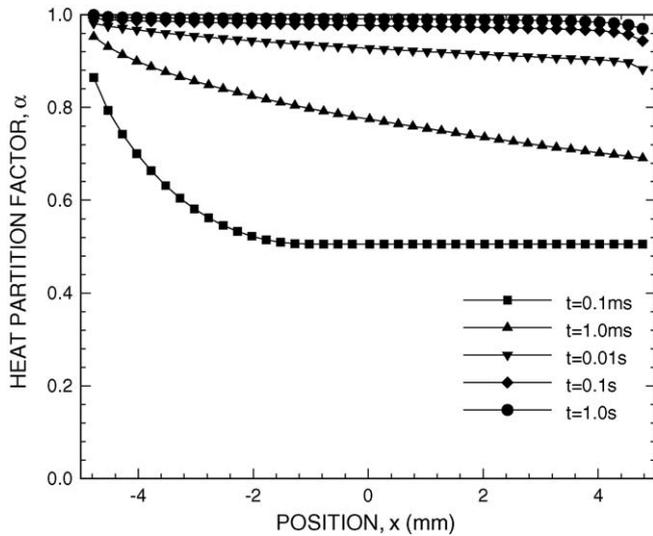
Fig. 2. Heat partition factor distribution along the contact patch at various times.
