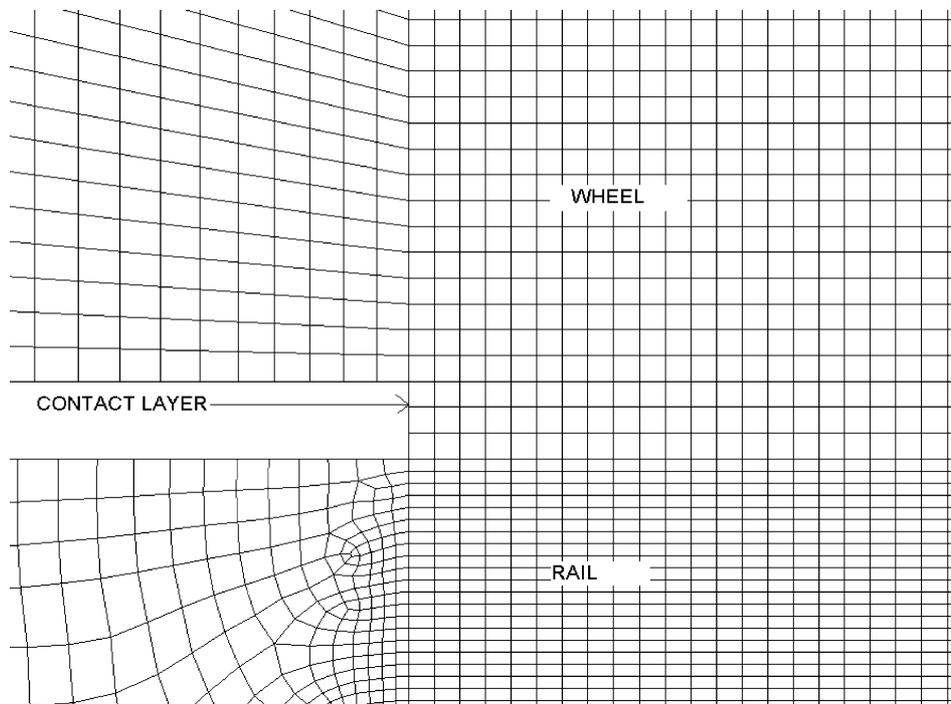
Fig. 1. Finite element mesh near the leading edge of the contact patch.
