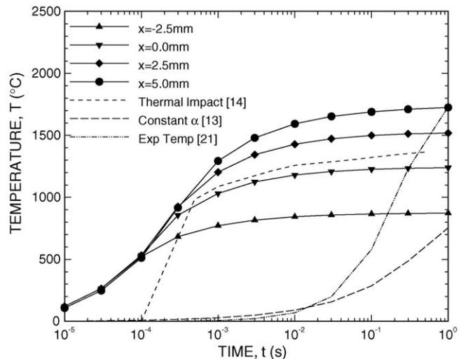
Fig. 5. Temperature vs. time at various positions along the contact patch.
