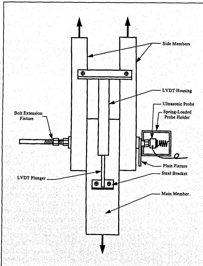
Figure 4 — Configuration for ultrasonic testing of bolts during connection tests.
