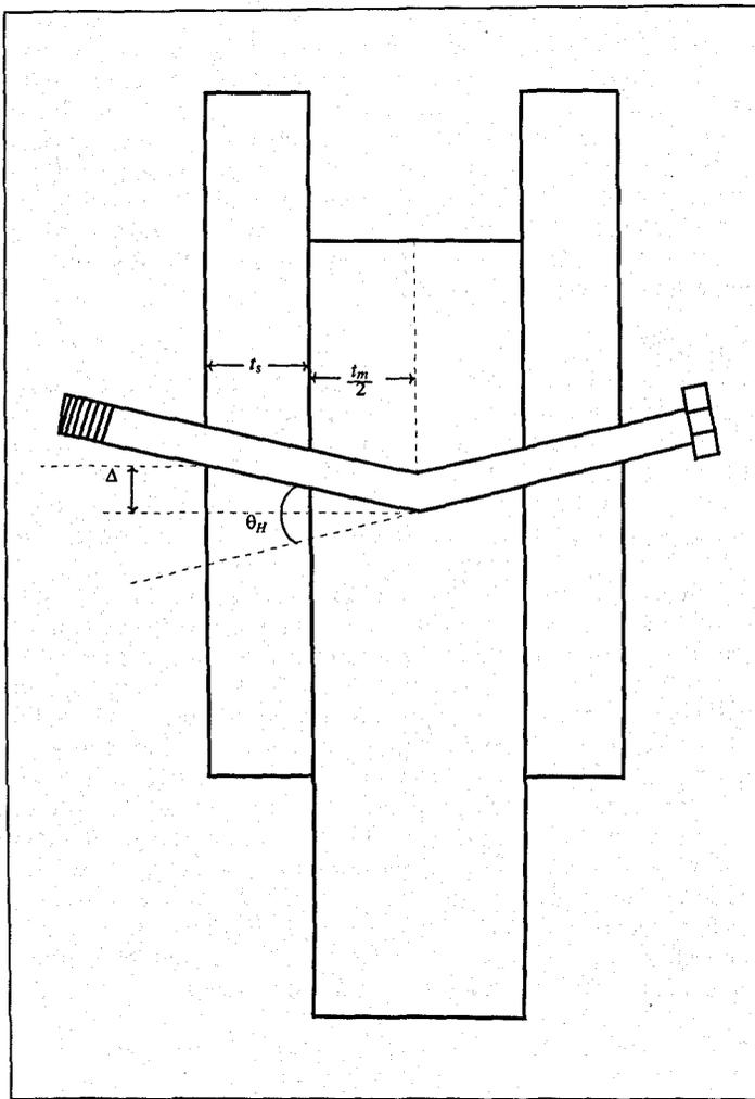
Figure 8 — Plastic hinge angle  $\theta_H$  for a bolt in a mode III, double shear connection.
