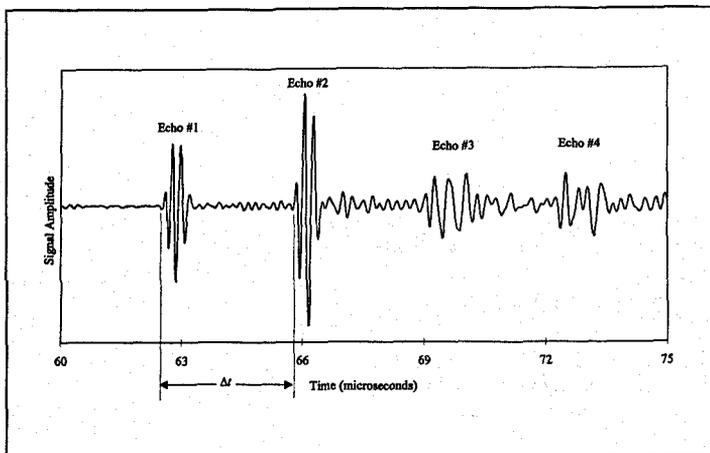
Figure 2 — Typical time domain signal for ultrasonic pulse echo testing of a straight bolt.
