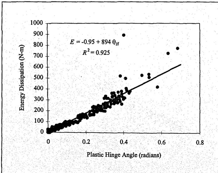
Figure 9 — Relationship between plastic hinge angle  $\theta_H$  and connection energy dissipation  $E$ .
