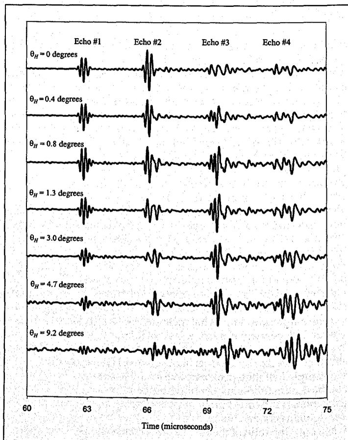
Figure 5 — Ultrasonic time domain signals for the testing of a 13 mm (0.5 in.) diameter bolt with a progressively increasing plastic hinge angle  $\theta_H$ .
