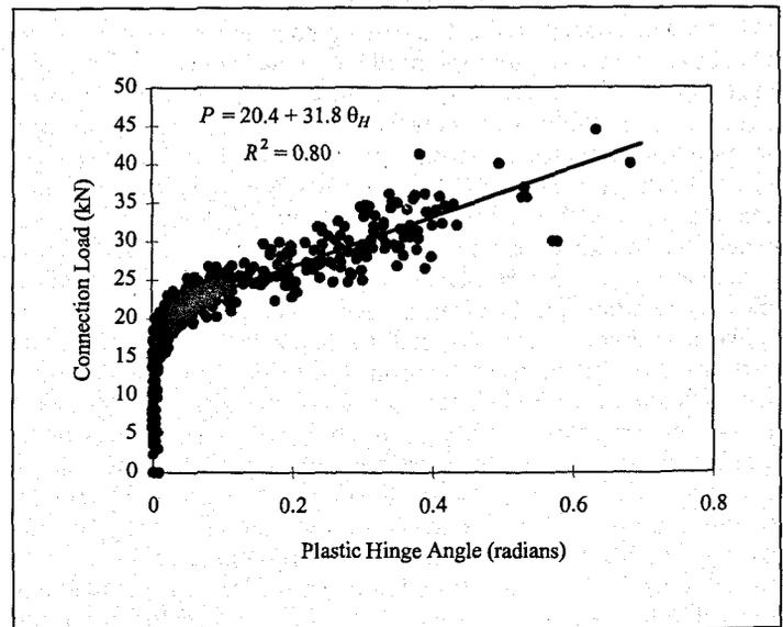
Figure 10 — Plastic hinge angle versus connection load; relationship between plastic hinge angle  $\theta_H$  and load beyond the connection yield point  $P$ .
