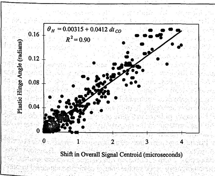
Figure 6 — Relationship between plastic hinge angle  $\theta_H$  and shift in ultrasonic signal centroid  $dt_{CO}$ .
