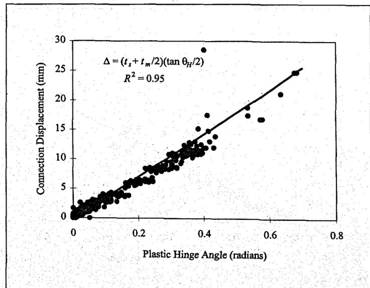
Figure 7 — Relationship between plastic hinge angle  $\theta_H$  and connection displacement  $\Delta$ .
