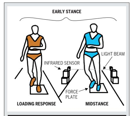
FIGURE 2. Subject at foot flat during the loading response and just before heel off, which is toward the end of midstance. The infrared photorelay used to trip the visual display is shown in background.
