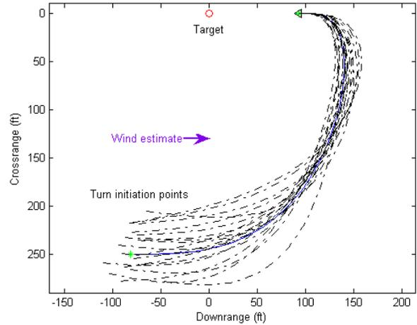
Fig.7 Optimal guidance with an error at TIP.
