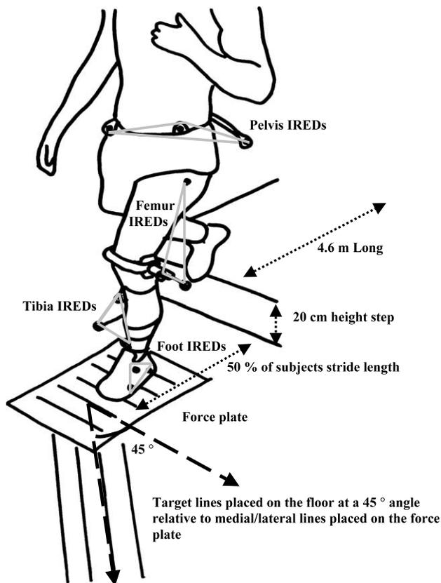
Fig. 1. The infrared emitting diodes for the four segment model of the lower extremity, arrangement of the step relative to the force plate and target lines used to help guide the subjects when performing the walk + cut and step + cut activities are illustrated.
