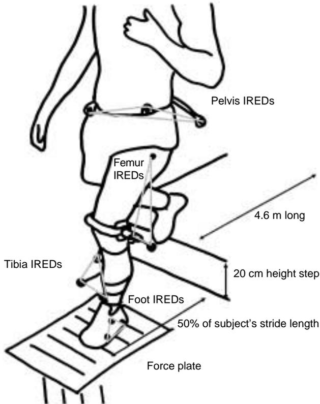
**FIGURE 1.** The placement of the infrared emitting diodes (IREDs) used to track lower extremity motion and placement of the step relative to the force plate. Each triangle represents the IREds used to track each segment of the 4-segment model.
