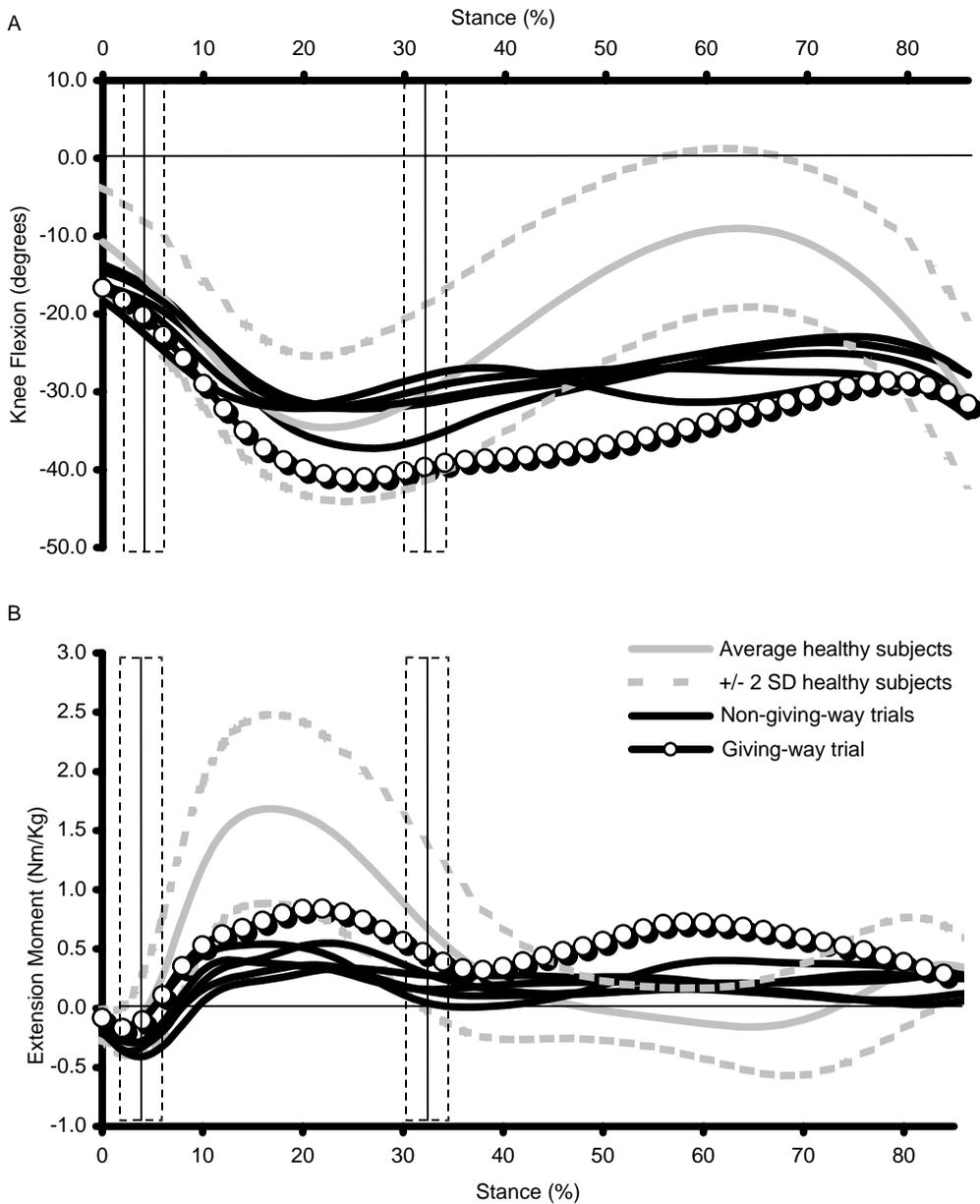
**FIGURE 3.** Knee flexion angle (A) and intrinsic knee extension moment (B) from 0% to 86% of stance for the healthy subjects, non-giving-way, and giving-way trials. The area between the vertical dashed lines (4% to 32%) indicates the period during stance when giving way took place (defined as a period of excessive tibial displacement).
