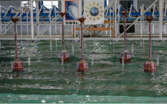
Fig. 1. Non-optimal array layout. Selected from literature search as a common array configuration.
