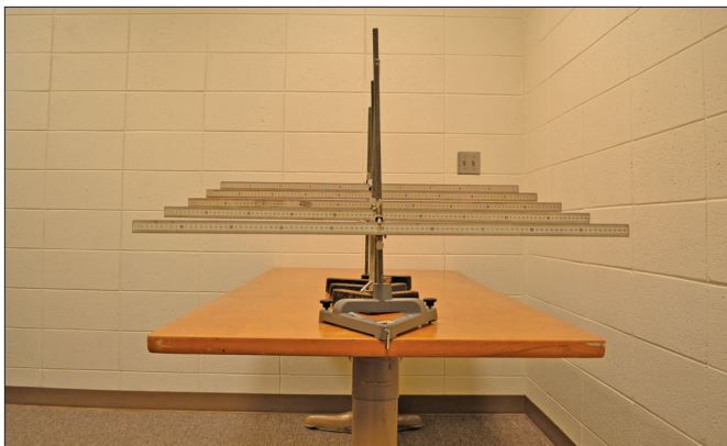
Fig. 2. Meterstick array used to study parallax.
